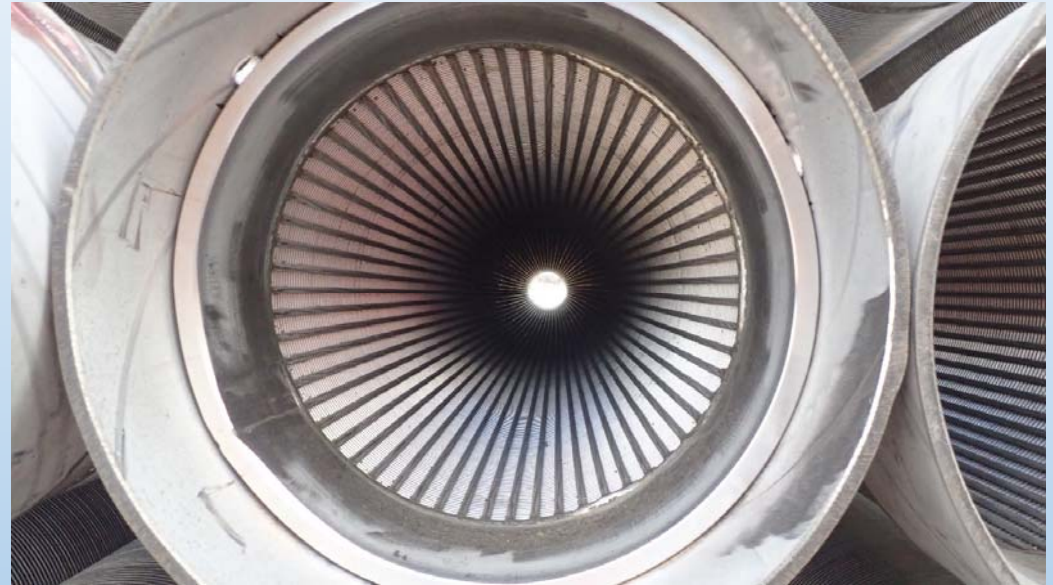
Well Screen from Stetson Engineers 2021 Well Drilling Project
